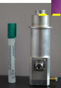
Elementary plasma source (design depending on the application)
